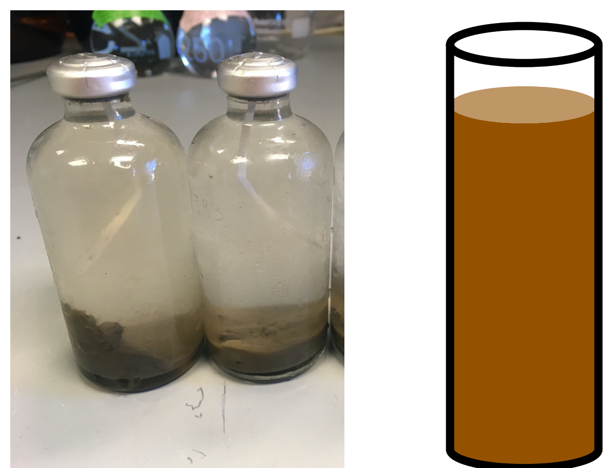
Fig 1. Example of a sediment slurry incubation (left) and the typical layout for an intact core sediment incubation (right).
